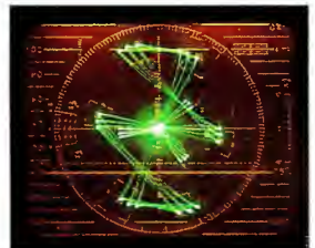
Triple Vector Overlay —SMPTE Bars on A, B and C inputs delayed by 6° and 12° to demonstrate phase error
