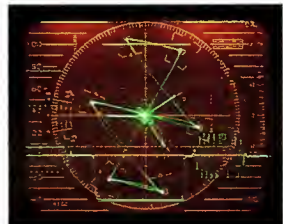
Combination Display —Simultaneous waveform and vector displays of a single input
